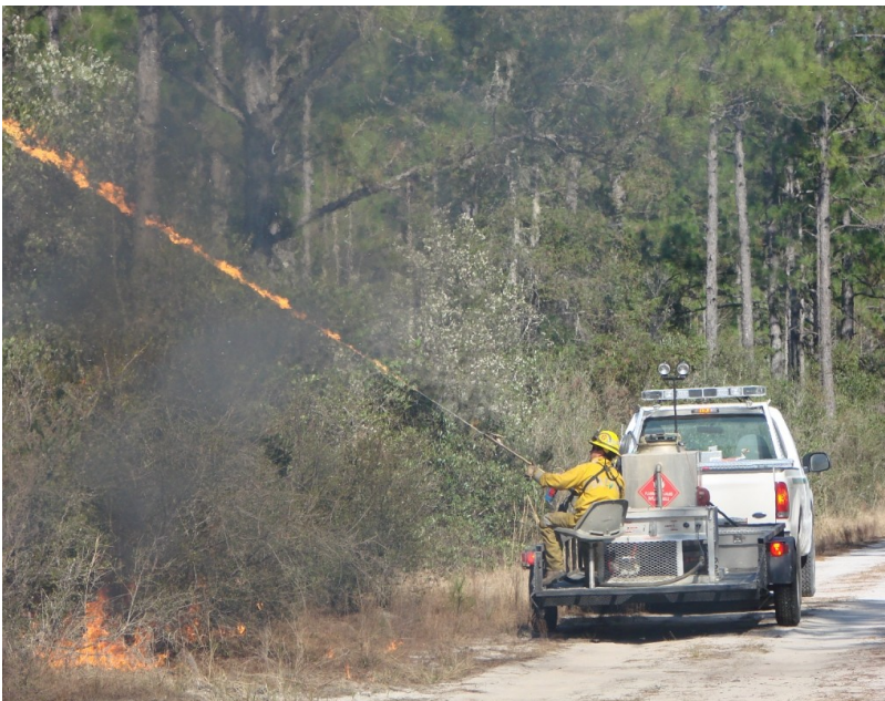
Flash21 can also be used with a Terra Torch for prescribed and back burning operations
